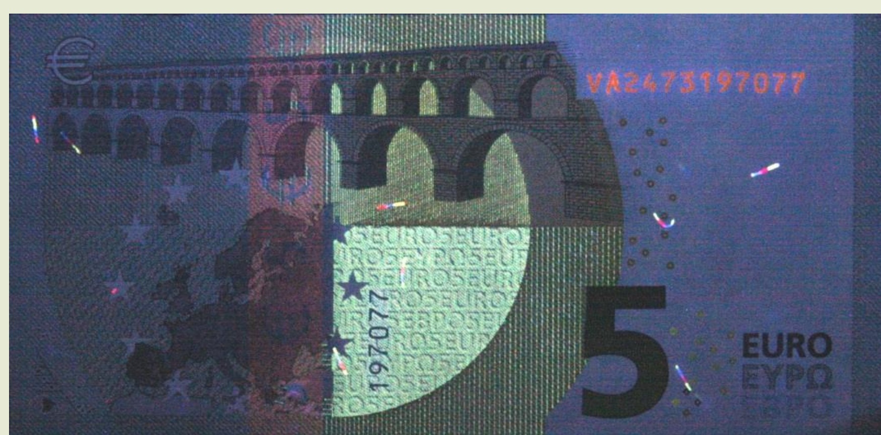
Figure 4: backside banknote, short-wave UV light
