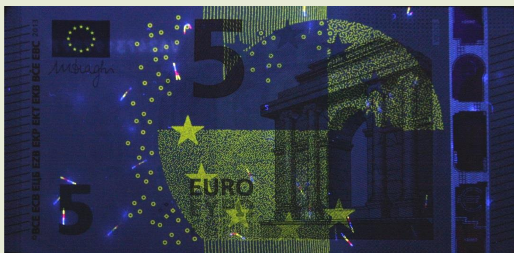
Figure 3: frontside banknote, long-wave UV light
